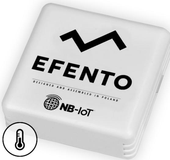
NB-IoT temperature sensors are used for remote temperature monitoring, in places where constant supervision is required, such as medical refrigerators, pharmaceutical wholesalers, museums, archives – especially suitable for monitoring distributed objects (transformer stations, pumping stations).
